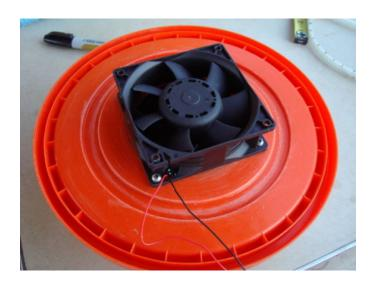
You can drill a small hole in the bucket lid to route the fan's power lines up thru the lid.
