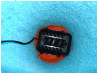
Install the the drip-line "lasso"; test fit so there's just a little slack from the pump to the top of the blue pad. Trim the excess hose, then connect the "lasso" to the pump nozzle:
