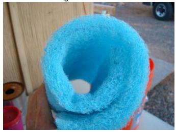
Slip the second smaller cylinder into the first blue cylinder, but not all the way in, leave the second cylinder about an inch popped out. This creates a double-layered pad with more evaporative surfaces:
