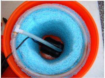
Guide the power lines from the pump up and out of the bucket. Cut a small notch at the rim of the bucket to route the power lines to the exterior of the bucket so the wires don't get kinked by when you put the lid on.
