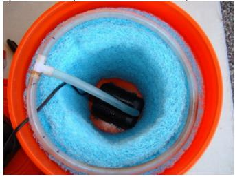
Cut the hose at the correct length, and plug in the T connector. Put a piece of leftover hose on the stem of the T-connector to complete the "lasso" (We will trim the excess hose later):
