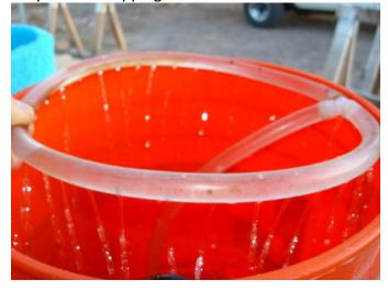
This is designed so that when the lid is put on, the drip line is gently pinched between the lid and the pad, so it stays secure.
