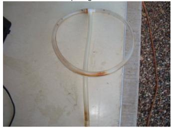
**T-Connector**: The branches of your T connector may be too long. Using a sharp exacto knife, cut off the excess branches, leaving approx ½ inch at each branch of the T connector. This creates a smaller joint for our project:
