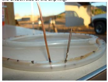
Get a candle and a thin piece of metal as a **piercer** (such as a thin nail or wire scrap. 12 gauge wire works well). A push-pin is a little too small but can work in a pinch. A power drill makes too jagged of a hole.
