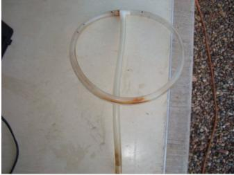
Now to create the drip holes, you will punch holes in the LOWER side of the drip-ring. So, remove the Lasso from the bucket, flip it over on the work table. Note that you are now working on the UNDER side of the drip ring:
