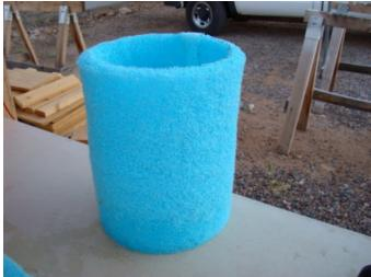
Cut a second piece of pad approx. 24x13 inches and roll into a tight tube. You don't need to glue or stich the seam of this small cylinder:
