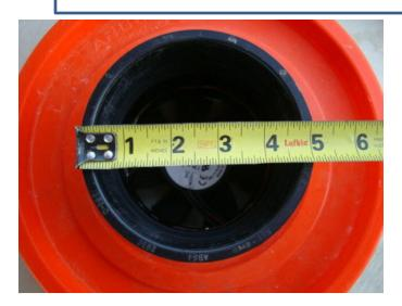
Mount the fan on the inside (ie bottom) of the bucket lid. Use the E6000 adhesive and short bolts/nuts to hold it in place. Slop some silicon sealer on any gaps. The fan woks best on the bottom of the lid to keep the unit compact and to make ducting easier. Having the fan on the inside also helps the blue pad hold its shape:
