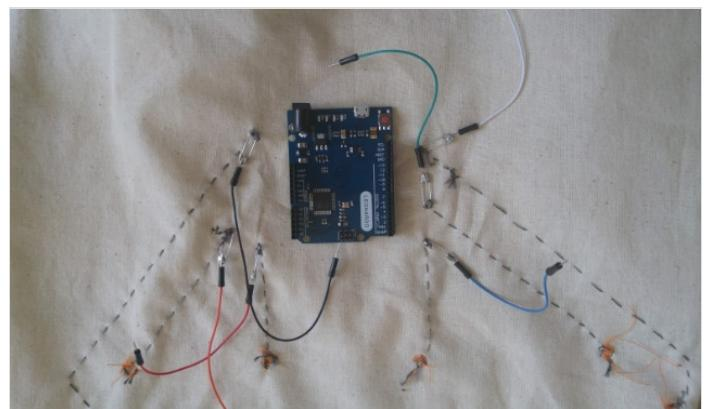
Étape 10 - Cover all safety pins with some tape to avoid short circuits and unwanted connections
